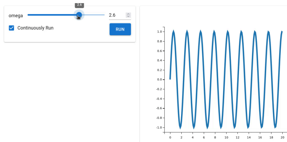
Figure 10. A sine wave generator with the autorun parameter toggled on. Source code in Program 16 .
