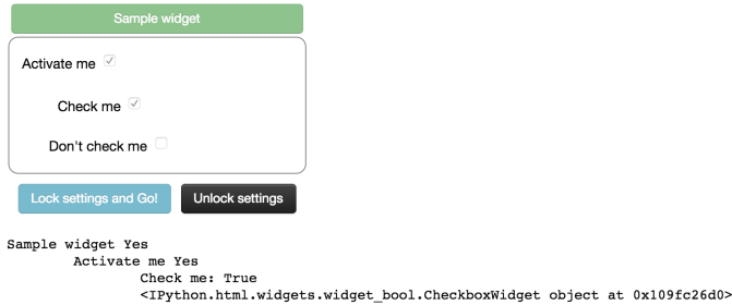
Fig. 6: The widget produced by the sample code in the section “reducer“ widget structure. Note the string output of the checkbox “Don’t check me”, whose __str__ method has not been overridden.
