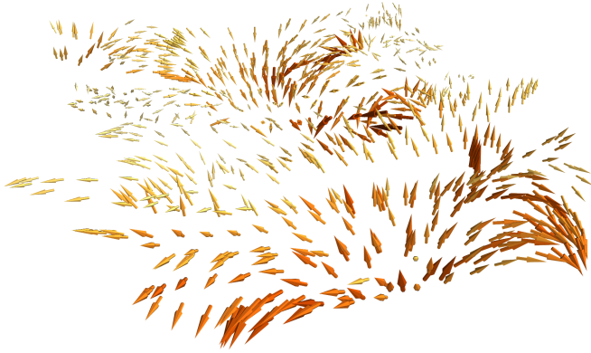
Fig. 3: Unstructured measurements of magnetic field distortion used to initialise an interpolated field model.
