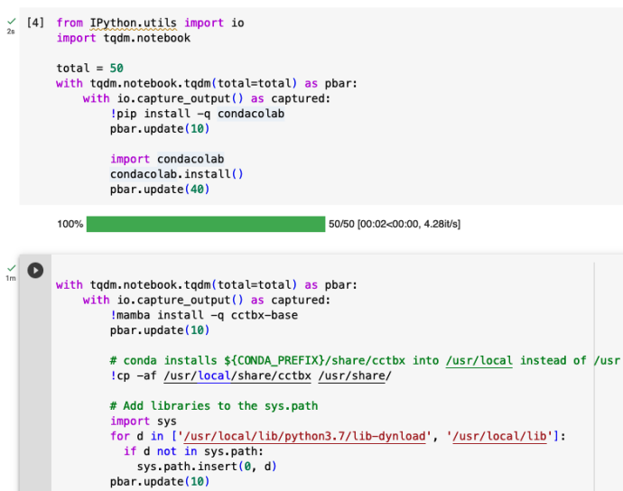
Fig. 7: Snippets from the cctbx library for installing mamba and then cctbx on Google Colab.
