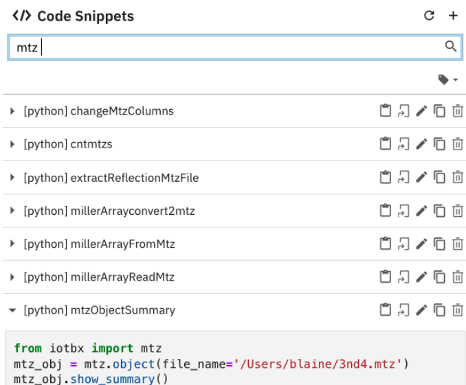
Fig. 5: Snapshot of a list of snippets in JupyterLab supported by the Elyra-snippet extension. The 80 cctbx snippets have been narrowed to seven snippets by entering the mtz tag. Additional tags can be entered to further narrow the list of candidate snippets.
