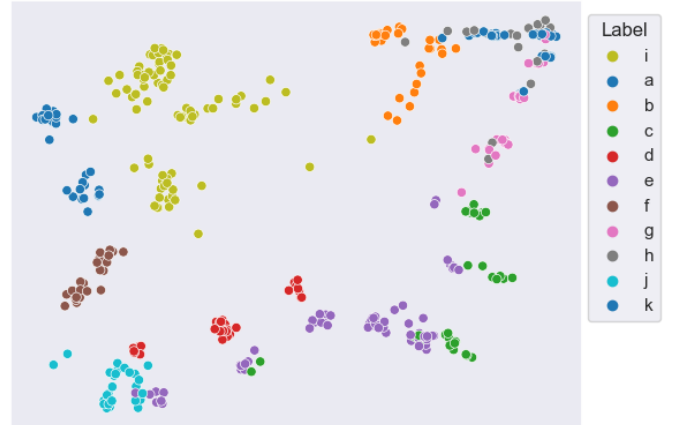
Fig. 6: Scatter plot showing syllables from the song of one Bengalese finch, embedded in a 2-D space using a convolutional encoder trained using the Parametric UMAP algorithm. Each marker is a point produced from a spectrograms of a single syllable rendition, mapped down to the 2-D space, from 40 seconds of training data. Colors indicate the label applied to each syllable by an expert human when annotating the spectrograms with a GUI.
